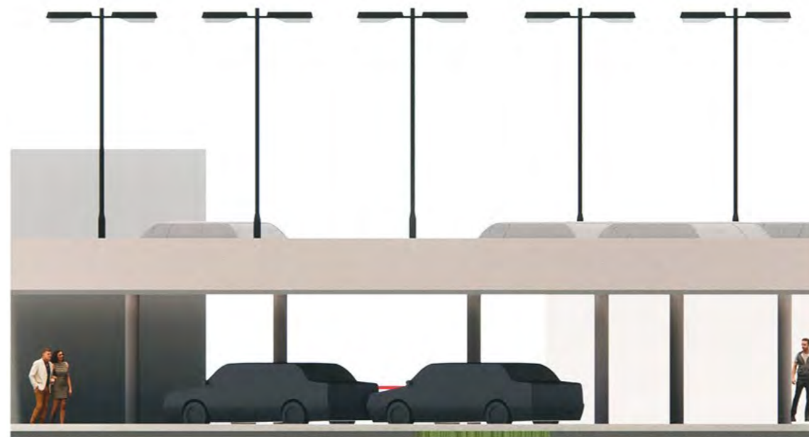
Figure 42. Indicative Elevation showing Typical 'Deck Parking' Design
